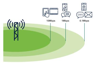
Figure 4 – Applications requirements in relation to network coverage
